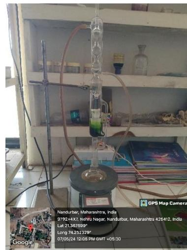
Fig 3: Extraction with Soxhlet Apparatus
